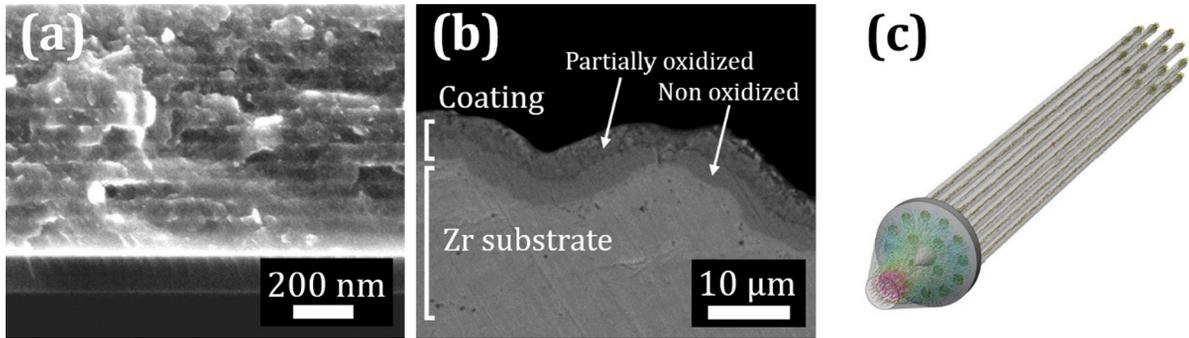
**Fig. 6.** Scanning electron microscope (SEM) cross-section (a) of a  $\text{CrC}_x/\text{CrN}$  multilayer coating grown by DLI–MOCVD constituted of 30 layers with a period of 53 nm, (b) of a protective  $\alpha\text{-CrC}_x$  coating after oxidation at high temperature as described in [18], and (c) computational simulation of a deposition in a bundle of 16 clad segments 1 m in length, validating the design of the gas-phase distributor.
