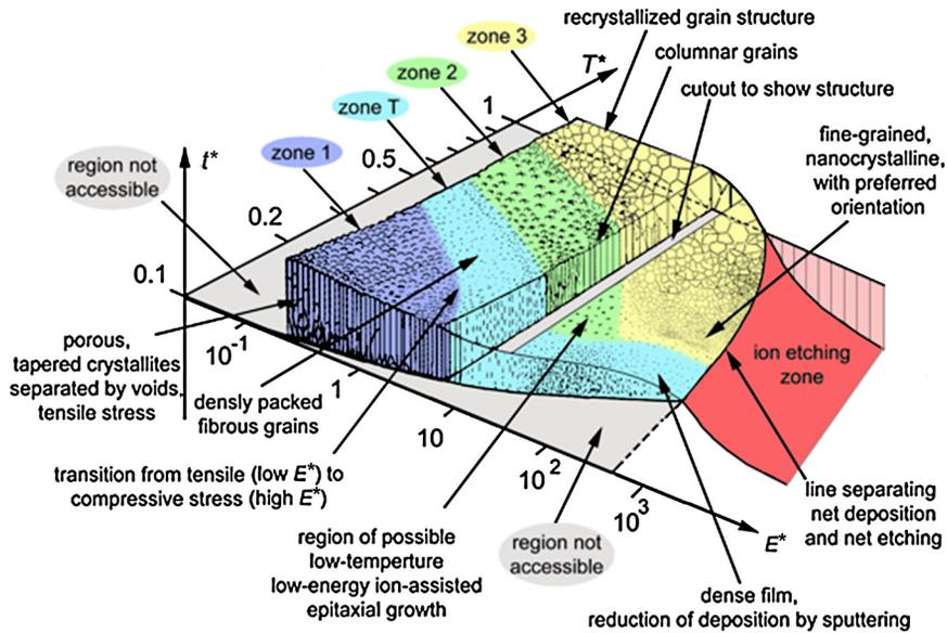
**Fig. 2.** Schematic morphology of coatings as a function of the generalized temperature ( $T^*$ ), which considers the temperature shift caused by the potential energy of the particles arriving on the surface, and normalized energy of impinging species ( $E^*$ ), which describes the displacement and heating effects caused by the kinetic energy of the bombarding particles, see Ref. [5] for an explanation (reproduced from [5]).
