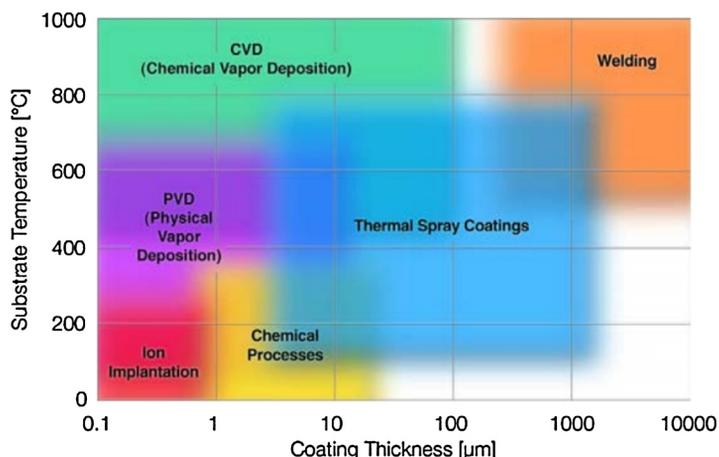
Fig. 1. Coating process comparison (reproduced from [1]).
