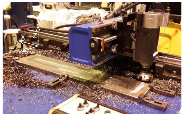
Fig. 1: Mobile machines for the cutting tests: machining robot and portable milling machine.
