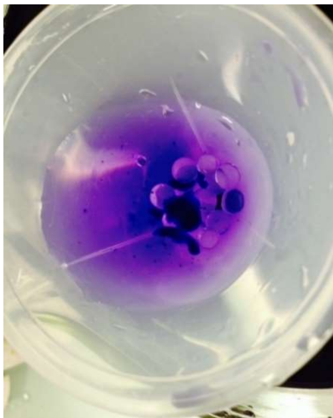
Fig. S-4: Chips of compacted cellulose 8%-175°C faces which were not fully dissolved after treatment: 6 \text{ g}\cdot\text{L}^{-1} (120 mg in 20 mL) for 24 h in 10 mL of water, 24 h in 10 mL of CED solution on a rotational shaker
