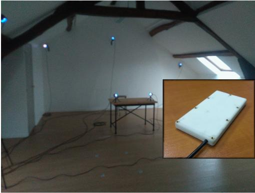
Fig. 2. Picture of the optitrack setup. The sensor board package is displayed in the insert.
