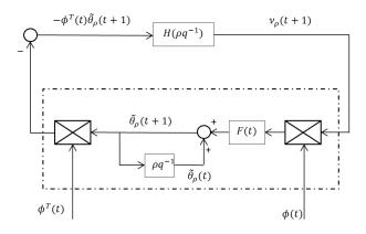
Fig. 2. Equivalent PAA closed-loop with  $\rho$ -signals
