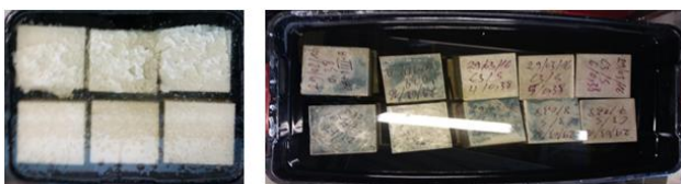
Figure 3 : Compressive strength of SCCs stored in 5% Na 2 SO 4 solution and water
