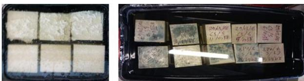
**Figure 4:** Left solution 5% H<sub>2</sub>SO<sub>4</sub>, right solution 5% Na<sub>2</sub>SO<sub>4</sub>
