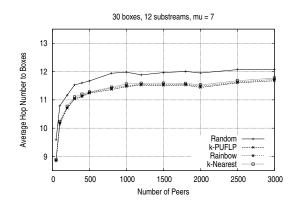
Fig. 3. Average distance (nb. of routers) when the number of clients increases
