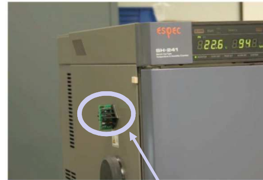
WPG-1 mounted vertically on side of oven
