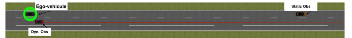
Figure 15: Scenario with a dynamic obstacle ( 16.5 m/s ) and a static obstacle. The ego-vehicle has an initial velocity of 25 m/s . The red curve represents the reference trajectory.
