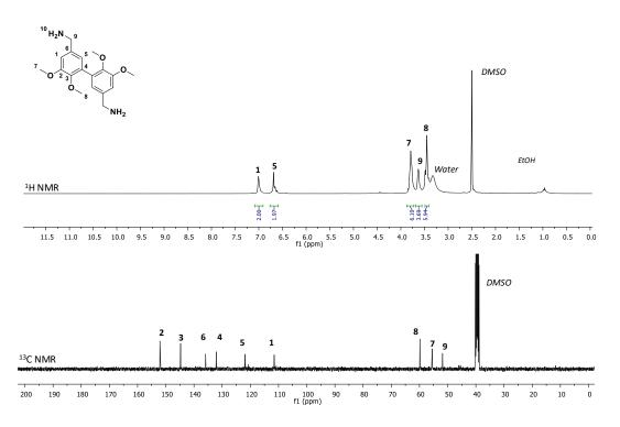
Figure 1: <sup>1</sup>H and <sup>13</sup>C NMR spectroscopy of methylated divanillylamine (MDVA) in DMSO-d6
