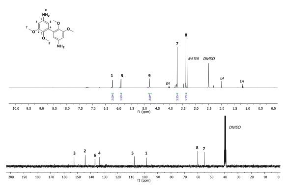
Figure 2: <sup>1</sup>H and <sup>13</sup>C NMR spectroscopy of 3,4-dimethoxydianiline (DMAN) in DMSO-d6
