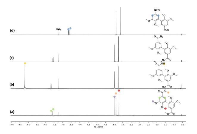
Figure S3 : <sup>1</sup>H NMR spectra of (a) methylated diester, (b) methylated divanillic acid, (c) methylated diacyl azide and (d) methylated di-isocyanate of vanillin in  $CDCI_3$
