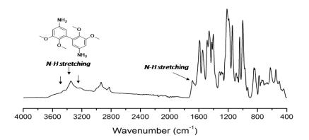
Figure S6 : FTIR spectrum of 3,4-dimethoxydianiline
