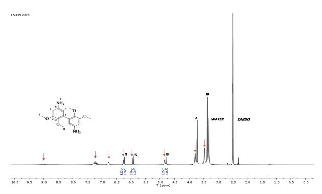
Figure S5: <sup>1</sup>H spectrum of 3,4-dimethoxydianiline before purification in DMSO-d6
