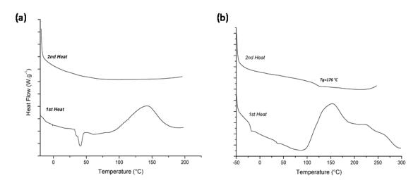
Figure S7 : DSC thermograms of (a) DGEBA/MDVA and (b) DGEBA/DMAN
