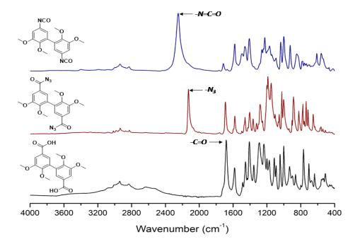
Figure S4 : FTIR spectra of methylated divanillic acid, di-acyl azide and di-isocyanate
