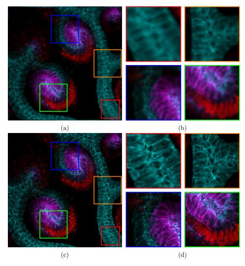
Figure 12: A restoration of images degraded by spatially varying blurs. The confocal image -  $512 \times 512$  - in Figure 3 has been blurred with the operator in Figure 11 and degraded with a noise level of  $5.10^{-3}$ . The pSNR of the degraded image (on top) is 22.3dB. Problem (2) is solved using the exact operator,  $\lambda = 10^{-4}$ , 500 iterations and Symmlet 6 wavelets decomposed 6 times. The pSNR of the restored image is 27.29dB.
