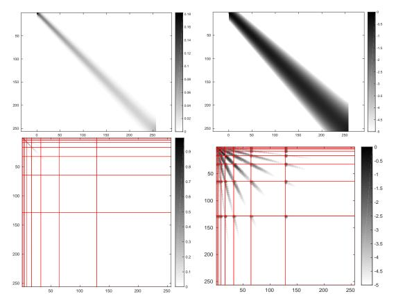
Figure 1: An illustration of the compression of a spatially varying blur in the wavelet domain. Top-left: H. Top-right: H in  $\log_{10}$ -scale. Bottom-left:  $\Theta$  obtained using Daubechies wavelets with 10 vanishing moments and a decomposition level J = 7. Bottom-right:  $\Theta$  in  $\log_{10}$ -scale.
