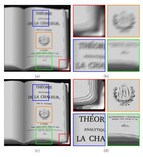
Figure 5: A deconvolution example. The book image in Figure 3 is blurred with the motion blur Figure 4b and degraded with a noise level of  $5.10^{-3}$ . The pSNR of the degraded image (on top) is 17.85dB. Problem (2) is solved using the exact operator,  $\lambda = 10^{-4}$ , 500 iterations and Symmlet 6 wavelets decomposed 6 times. The pSNR of the restored image is 24.14dB.
