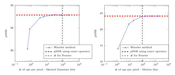
Figure 8: Evolution of the pSNR of the deconvolved image w.r.t. the number of operations per pixel per iteration. The gray vertical line gives the number of operations per pixel per iteration to solve the exact  $\ell^1$ -problem 2 using FFTs and FWTs. The horizontal line gives the pSNR obtained using the exact operator.
