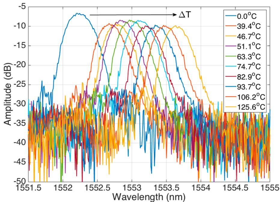
Figure 4. Reflection spectra of the MgO-NP FBG, for different values of temperature variation  $\Delta T$ ; the reference temperature  $\Delta T = 0^\circ\text{C}$  corresponds to room temperature.
