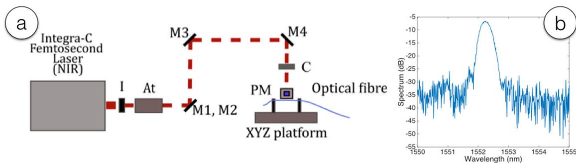
**Figure 1.** (a) Schematic diagram of the laser inscription setup used to inscribe refractive gratings; I—iris, At—power attenuator, M—mirror, C—Convex cylindrical lens, PM—Phase mask. (b) Spectrum of the FBG inscribed on the MgO-NP having Bragg wavelength around 1552.2 nm.
