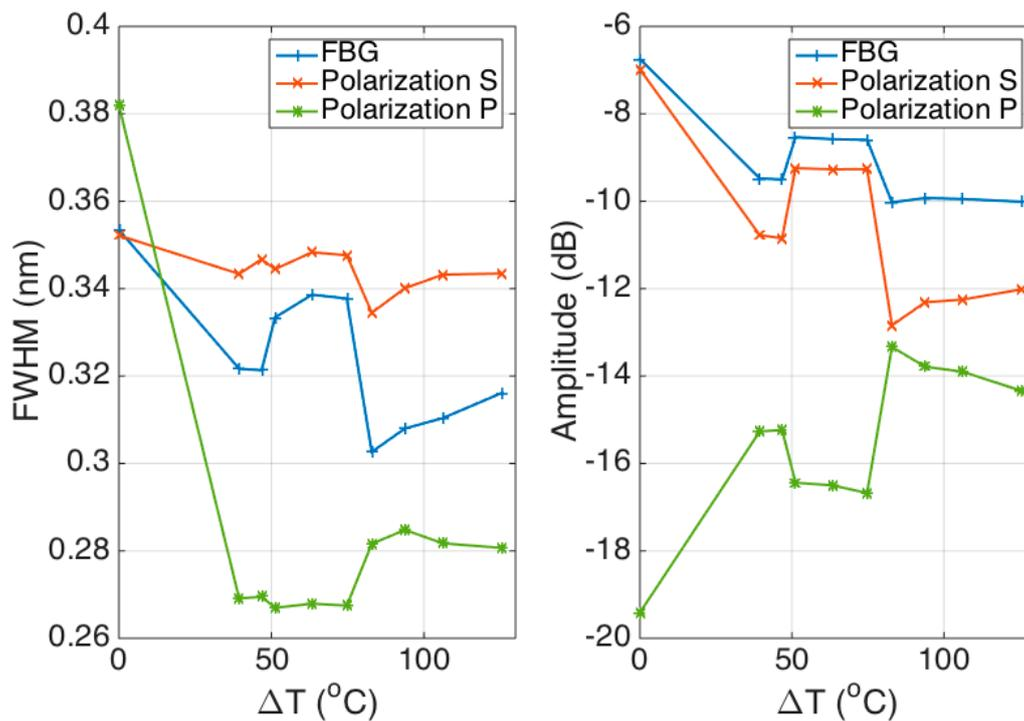
**Figure 8.** Polarization analysis of the FBG parameters: the chart reports the FWHM (**left**) and the maximum amplitude (**right**) of the FBG spectra at different temperature values, for the whole FBG and for each polarization independently.
