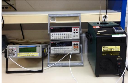
Figure 6 Calibration test bench.
