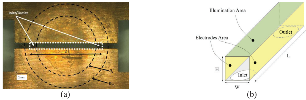
Figure 2: a) Optical microscope image indicating microchannel, illumination and window diameters; b) Microchannel schematics with main geometry and geometrical parameters.
