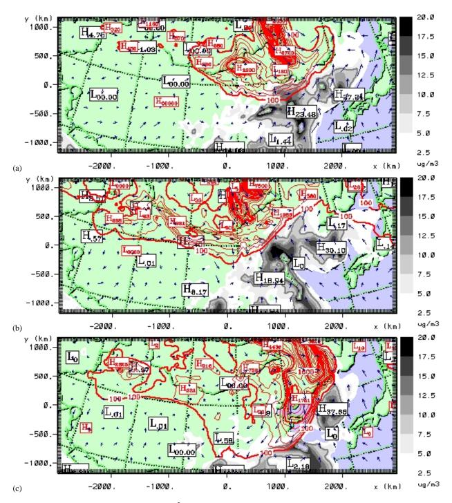
**Fig. 6.** Modelled surface BC concentrations (in  $\mu$ g m<sup>-3</sup>, grey-coloured contours and black labels: H stands for maximum; L for minimum), and modelled surface dust concentrations (in  $\mu$ g m<sup>-3</sup>, red-coloured contours and labels) at 00:00 UTC (08:00 LT). Blue arrows represent surface winds (a. u.): Results on 28 April (**a**), 30 April (**b**) and 1 May (**c**), 2005.
