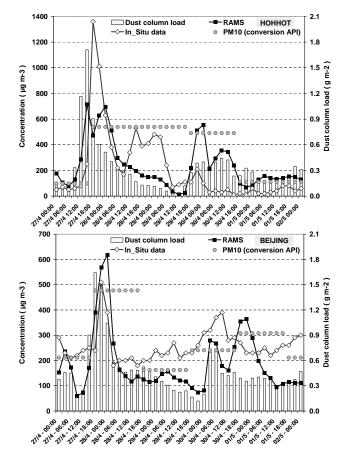
**Fig. 10.** Time series of the surface mineral dust concentrations (in  $\mu g m^{-3}$ ) and of the vertical integrated column load (in  $g m^{-2}$ ) over Hohhot (**a**) and Beijing (**b**): modelled concentrations (black squares); *in situ* observed concentrations (diamonds); PM<sub>10</sub> concentrations from API data (grey circles) and modelled column loads (bar charts).
