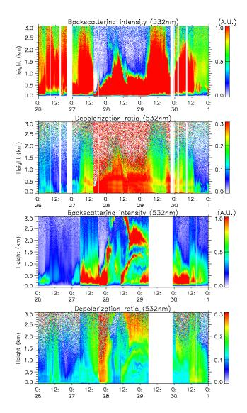
**Fig. 12.** Lidar measurements (532 nm) from 26 April 2005, 00:00 UTC to 1 May 2005, 00:00 UTC at Hohhot (upper group of two figures) and Beijing (lower group of two figures). For each group: – higher part: backscattering intensities (a. u.) – lower part: depolarisation ratio.
