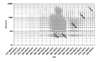
**Fig. 9.** Symbolic intercomparison of the "captured" SO<sub>2</sub> concentrations (grey spheres): time series (UTC) of the vertical distributions (altitudes: logarithmic scale) over Beijing.
