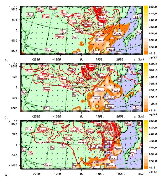
**Fig. 7.** Modelled surface SO<sub>2</sub> concentrations (in  $\mu g m^{-3}$ , orange-coloured contours and brown labels: H stands for maximum; L for minimum), and modelled surface mineral dust concentrations (in  $\mu g m^{-3}$ , red-coloured contours and labels) at 00:00 UTC (08:00 LT). Blue arrows represent surface winds (a. u.): Results on 28 April (**a**), 30 April (**b**) and 1 May (**7**), 2005.
