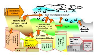
**Fig. 3.** Summary of the atmospheric processes undergone by sulphur compounds, mineral dust and BC accounted for in the simplified model over polluted areas.
