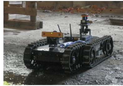
FIGURE 2: RAPOSA-NG, a tracked wheel search and rescue UGV prototype.
