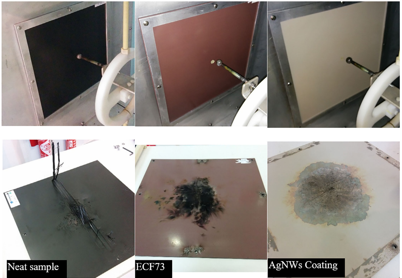
Figure 9. Nonimpacted (top) and impacted (bottom) samples without LSP (right), with ECF73 (center) and with AgSWs coating 8% in volume. [Color figure can be viewed at wileyonlinelibrary.com ]
