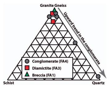
FIG. 4.—Ternary diagram (schist-granite gneiss-quartz) showing the composition of the breccia (FA1), diamictite (FA3), and conglomerate (FA4).
