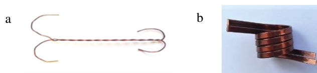
Fig.1. Specimens: a – twisted pair, b - coil
