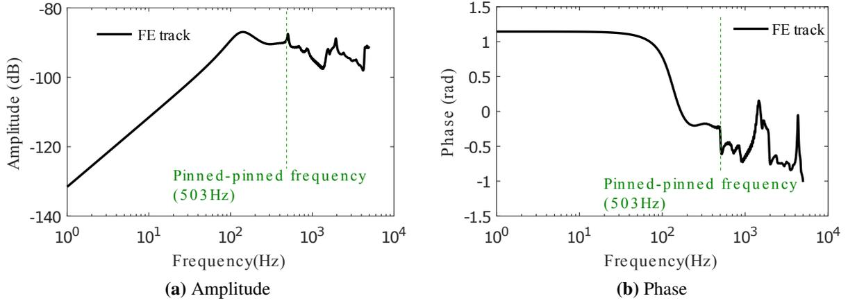
**Figure 8:** Lateral mobility at contact point (Reference amplitude: 1 m/s/N)
