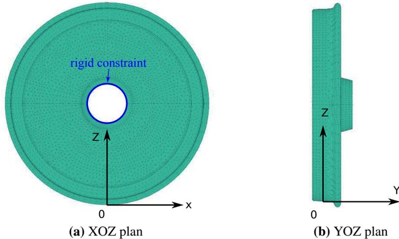
**Figure 3:** Wheel FEM mesh (wheel of type "Vyksa BA005" with a nominal rolling diameter of 920 mm and a mass of 314 kg) with a rigid constraint applied at the inner face of the hub, where the wheel is connected to the axle.
