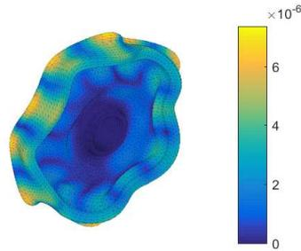
**Figure 11:** Unstable mode shape with the rigid track
