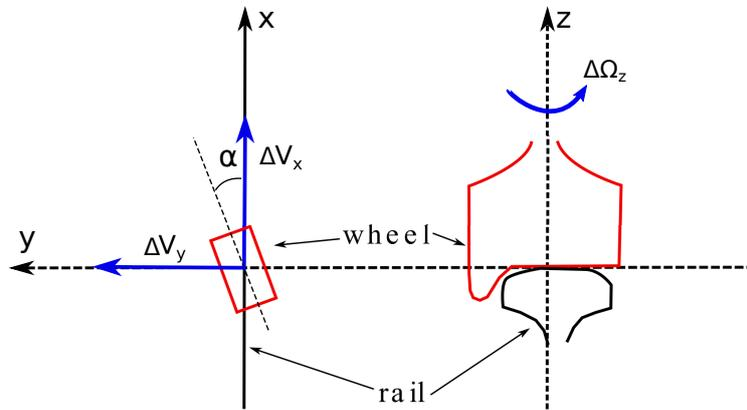
**Figure 2:** Coordinate system, kinetic variables ( $\alpha$ : angle of attack of the curve,  $\Delta V_y$ : imposed lateral sliding velocity,  $\Delta V_x$ : imposed longitudinal sliding velocity and  $\Delta \Omega_z$ : imposed spin velocity)
