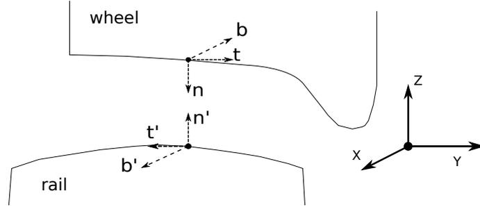
**Figure 1:** Reference frame of the wheel/rail interaction. The rolling direction along the rail is the  $x$ - direction. The lateral direction is the  $y$ - direction. The vertical direction is the  $z$ -direction.  $(n, t, b)$  and  $(n', t', b')$  are respectively the local frames of the wheel and the rail such that:  $n' = -n = Z$ ,  $t' = -t = -Y$ ,  $b' = -b = X$
