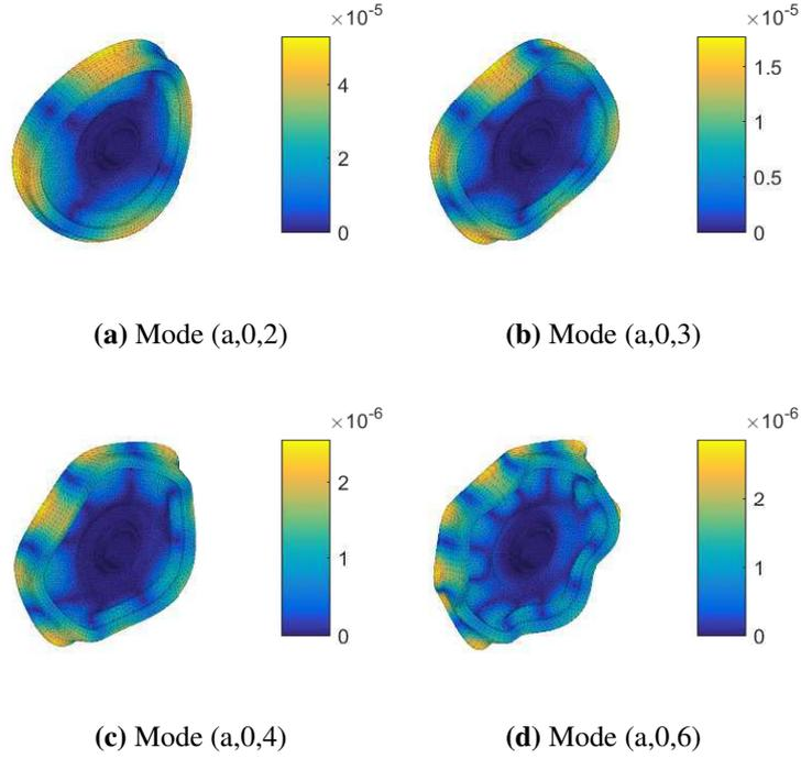
**Figure 13:** Unstable modes shapes with the flexible track
