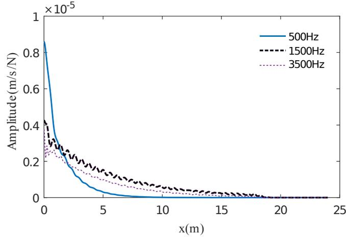
**Figure 9:** Vertical mobility along the track caused by the impulsion at the contact point ( $x = 0$ )
