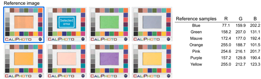
Figure A10. Constitution of a CaliPhoto database of coloured paper. Reference image used for the CaliPhoto image processing correction and corrected images of the reference samples. The areas corresponding to the samples are selected, and the average colours are calculated and stored in a database, as shown in the table.
