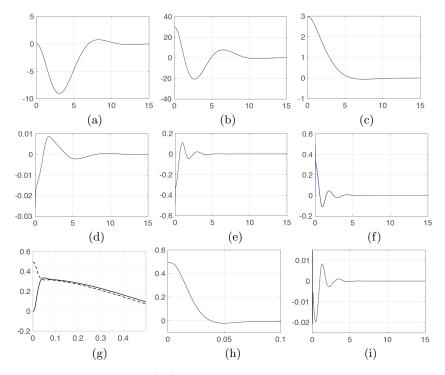
Figure 5: Nonlinear description (1.2) controlled by the robust asymptotic feedback linearization (1.3), (1.11) and (3.8). (a)  $\times$  [m], (b)  $\theta$  [°], (c) z [m], (d)  $u_x$  [kg m s<sup>-2</sup>], (e)  $q_{x,*}(x)$  [s<sup>-2</sup>], (f) and (g)  $q_{x,*}(x)$  (dash line) vs  $\bar{u}_x$  (solid line) [rad s<sup>-2</sup>], (h) and (i)  $q_{x,*}(x) - \bar{u}_x$  [rad s<sup>-2</sup>].
