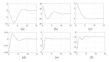
Figure 4: Nonlinear description (1.4) controlled by the usual exact feedback linearization (1.3) and (1.17). (a)  $\times$  [m], (b)  $\theta$  [°], (c) z [m], (d)  $u_x$  [rad kg m s<sup>-2</sup>], (e)  $\alpha(x)$  [m s<sup>-4</sup>], (f)  $\beta(x)$  [m rad<sup>-1</sup> s<sup>-2</sup>],
