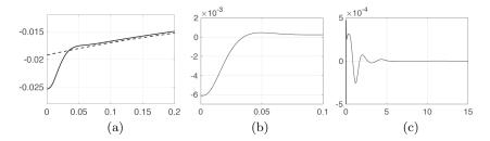
Figure 6: Comparison of control outputs  $u_x$  obtained in both simulations. (a)  $u_x$  from Figure 4 (obtained with the exact feedback linearization (1.3) and (1.17); dash line) vs  $u_x$  from Figure 5 (obtained with the robust asymptotic feedback linearization (1.3), (1.11) and (3.8); solid line) [rad kg m s<sup>-2</sup>], (b) and (c) Difference of the control signals  $u_x$  issued from Figures 4 and 5.
