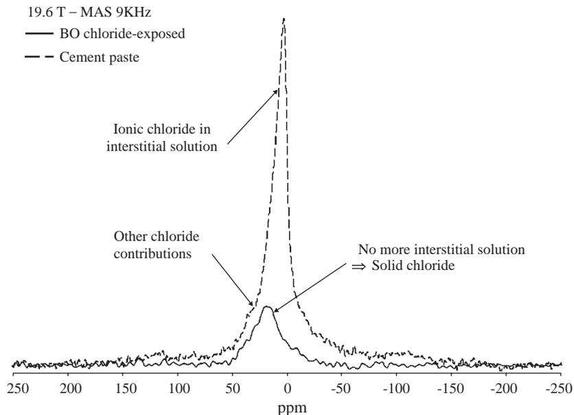
Fig. 5.  $^{35}\text{Cl}$  spectra of the concrete BO chloride-exposed sample (full line) and the cement paste (dash line) at 19.6 T. The cement paste spectrum is the superposition of one peak near 0 ppm (ionic chloride) and another one near 30 ppm (solid or adsorbed chloride). The concrete spectrum exhibits only the solid (attributed to Friedel's salt) and the adsorbed chloride contribution.
