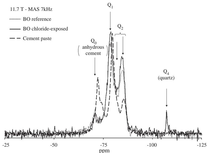
Fig. 3.  $^{29}\text{Si}$  spectra of the BO reference concrete (dot line) and the chloride-exposed sample (full line) at 11.7 T. The comparison between the chloride-treated and the reference samples shows a rehydration of previously unreacted anhydrous cement due to the chloride exposure.
