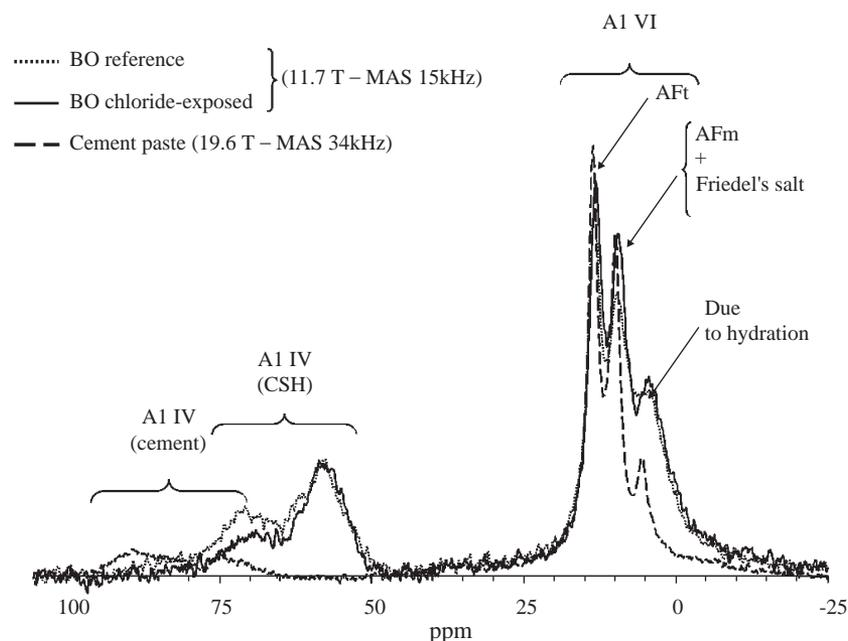
Fig. 4.  $^{27}\text{Al}$  spectra of the concrete BO reference sample (dotted line) and the chloride-exposed sample (full line) at 11.7 T and the  $^{27}\text{Al}$  spectrum of the cement paste (dash line) at 19.6 T. Exposure to chloride leads to the formation of Friedel's salt. Al IV modifications appear when the concrete is in contact with a saline solution. Al IV for the cement present only the characteristic of aluminum incorporated in the cement.
