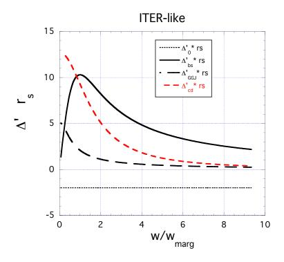
FIG. 2. Terms in the Rutherford equation (9) vs.  $w/w_{marg}$  for m=2, n=1 NTM in ITER-like scenarios. Classical  $\Delta'_{0J}$  (dotted line); neoclassical bootstrap effect  $\Delta'_{bsJ}$  (full line); toroidal  $\Delta'_{GGJ}$  (long dashed line); helical driven current  $\Delta'_{CD}$  (short dashed line) [12].
