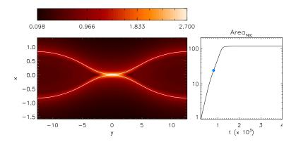
FIG. 6. Left frame. Contour plots of the current density at the time  $t_1 = 800$ , when the ECCD starts to be injected. The superimposed white lines identify the borders of the corresponding magnetic island. The right frame shows the time evolution of the magnetic island area in absence of ECCD control.
