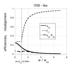
FIG. 5. (left) ECCD efficiency vs.  $w/w_{cd}$  for CW(full line) or 50% modulation (dashed line) of  $J_{CD}$ , perfectly phased and radially aligned on O-point [14]; (right) plots of  $\eta_{CDm.n}$  (full line)), $G_{CD}$  (thin-dashed line) and  $\eta_{CDm.n}G_{CD}$  vs.  $w/w_{cd}$  (thick-dashed line) for a radial misalignment  $\delta R = 0.016m$  considering a 2/1 NTM.
