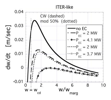
FIG. 4. NTM phase space dw/dt vs w; example of control of m=2, n=1 NTM magnetic island width down to the self-extinguishing value, by perfectly phased  $J_{CD}$  injection in an ITER-like scenario, showing the difference between CW ( $0 \le P_{EC} < 4.1 MW$ ) and 50% modulated case CW ( $0 \le P_{EC} < 3.7 MW$ ).
