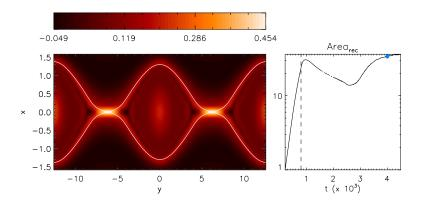
FIG. 7. Left column, from top to bottom. Contour plots of the current density in presence of ECCD beams of width  $w_{cd} = b[\psi_X - \psi_O]$  with b = 0.5, 1, 2. The superimposed white lines identify the borders of the corresponding reconnected region. The right column shows the time evolution of the area of the reconnected region for the three cases. The dashed lines identify the starting injection time  $t_1 = 800$ , while the blue dots show the time when the current is plotted.
