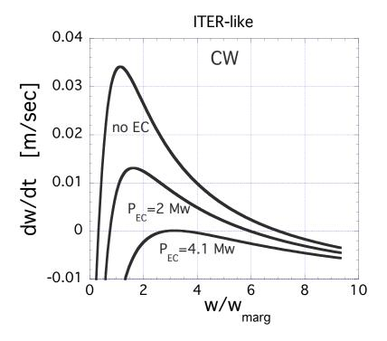
FIG. 3. NTM phase space dw/dt vs.  $w/w_{marg}$  for an NTM 2/1. The effects of different values of  $J_{CD}$  using CW EC power injection for an ITER-like scenario are shown. The mode is suppressed by 4.1 MW of EC power for  $w_{cd}$  width =0.04 m.
