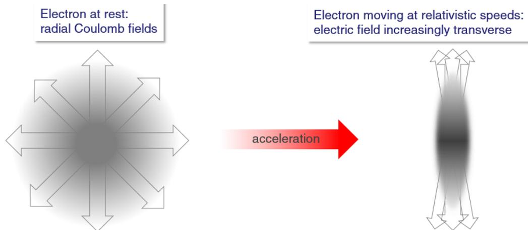
**Figure 3.** The electric field of a point charge in the lab frame is mainly transverse, scaling with its Lorentz factor  $\gamma$ .
