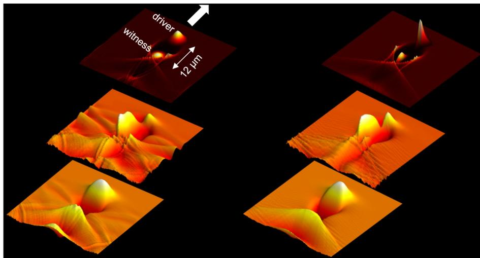
**Figure 7.** An electron double bunch from an LWFA stage is put into a second, higher density plasma stage, where it acts as a driver-witness pair PWFA energy afterburner. The right hand side shows a later snapshot during the PWFA acceleration, where plasma lensing has pinched both driver and witness bunch. The top plots shows the electron density, the middle plots the transverse electric field, and the bottom plots show the longitudinal wakefields. Visualization adapted from [4].
