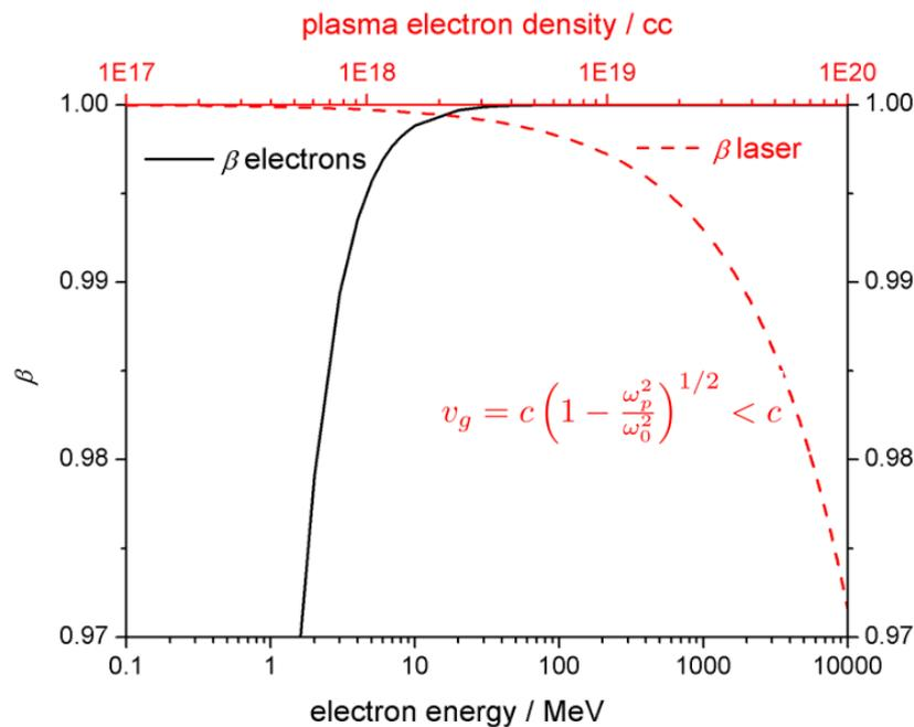
**Figure 5.** The velocity of electrons in plasma is independent of plasma density, while the laser pulse group velocity in plasma decreases with increasing plasma density. Electron velocities in terms of corresponding  $\beta$  are plotted in black vs. electron energy, while the laser pulse group velocity is plotted in red vs. plasma density.
