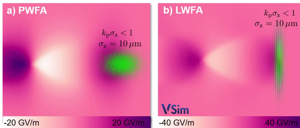
**Figure 1.** PIC-simulation visualization of electron-driven PWFA (a) and laser-driven LWFA (b) in the blowout/bubble regime, respectively. The driver beam is shown in green and propagates to the right, expels plasma electrons (not shown) and thus generates strong trailing electric decelerating/accelerating fields.
