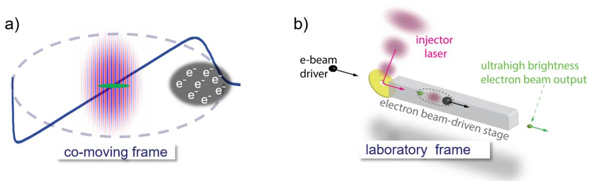
**Figure 10.** (a) Collinear Trojan Horse schematic in the co-moving frame; and (b) laboratory frame. The laser focusing pulse releases ultracold electrons (green) from the high ionization threshold medium, which then briefly fall back and are trapped in the back part of the accelerating blowout.
