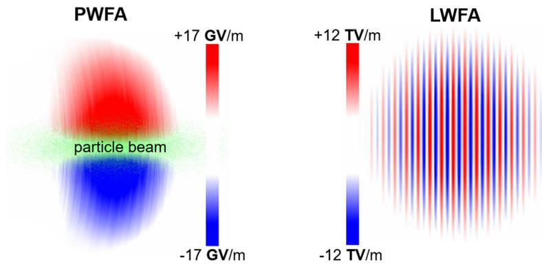
**Figure 4.** The electric fields of electron bunch PWFA drivers are unipolar, while electric fields of laser pulse LWFA drivers are oscillating. As a result, the peak electric fields, which are required to excite a similarly strong blowout/bubble, are three orders of magnitude lower for PWFA than for typical LWFA Ti:sapphire lasers.
