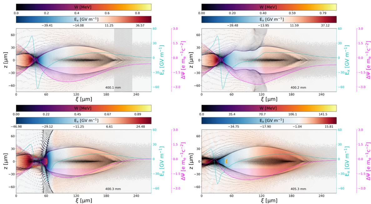
**Figure 9.** Plasma torch injection in PIC-simulations with VSim. The drive beam (black) propagates to the right and drives a plasma wave based on preionized hydrogen. A laser pulse has generated a helium-based plasma torch perpendicular to the drive beam propagation axis, constitutes a density ramp and triggers density downramp injection.
