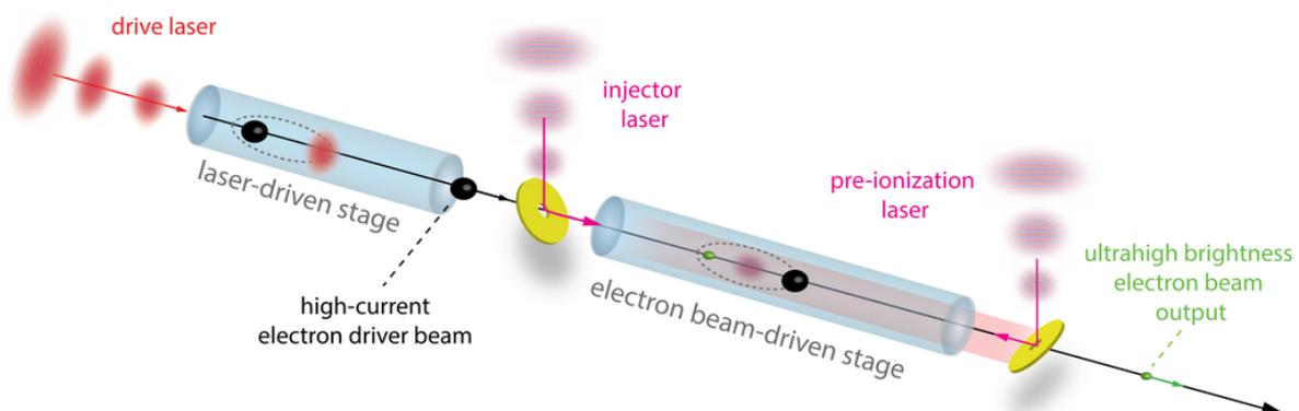
**Figure 11.** Potential setup of a “triple-hybrid” system where the laser system generates the electron bunch driver for PWFA via LWFA, is used to preionize the PWFA stage, and for witness bunch generation via the Trojan Horse mechanism.
