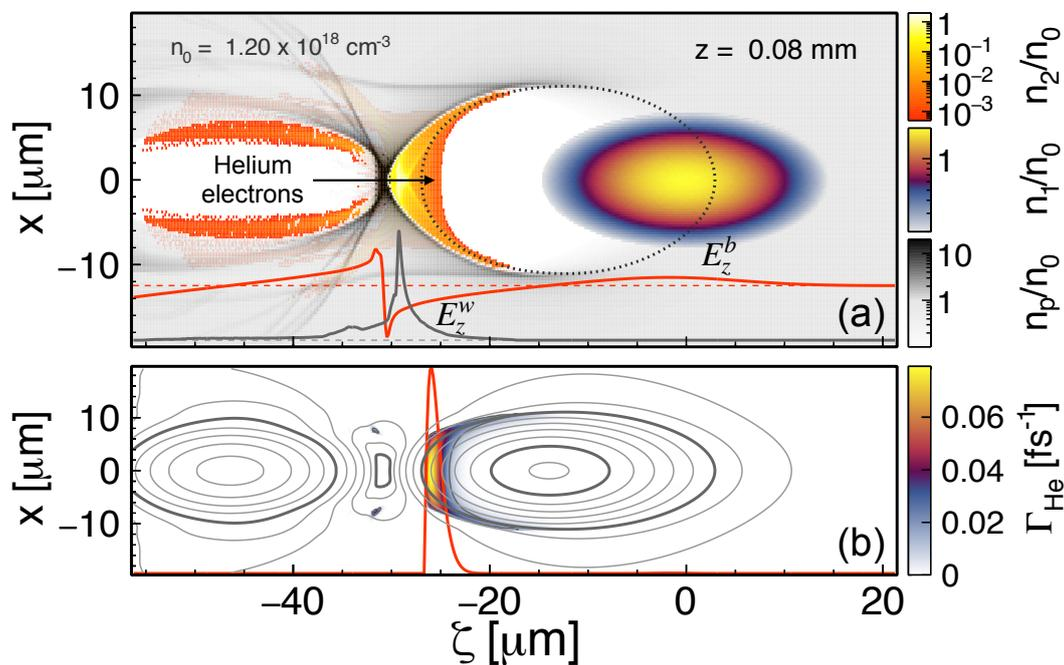
**Figure 12.** OSIRIS 3D simulation of a PWFA with WII injection: (a) electron density of the drive beam, the plasma and the ionized helium; and (b) ionization rate for He according to the ADK model. The contours in (b) show the wakefield-equipotential surfaces in steps of 0.2.
