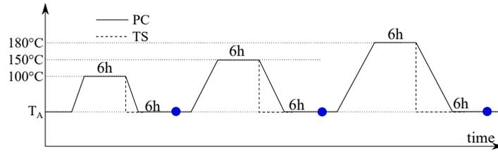
**Figure 2** The two considered thermal treatments. PC stands for Progressive Cooling and TS for Thermal Shocks. Blue dots represent the measurements performed after 6 h of cooling.
