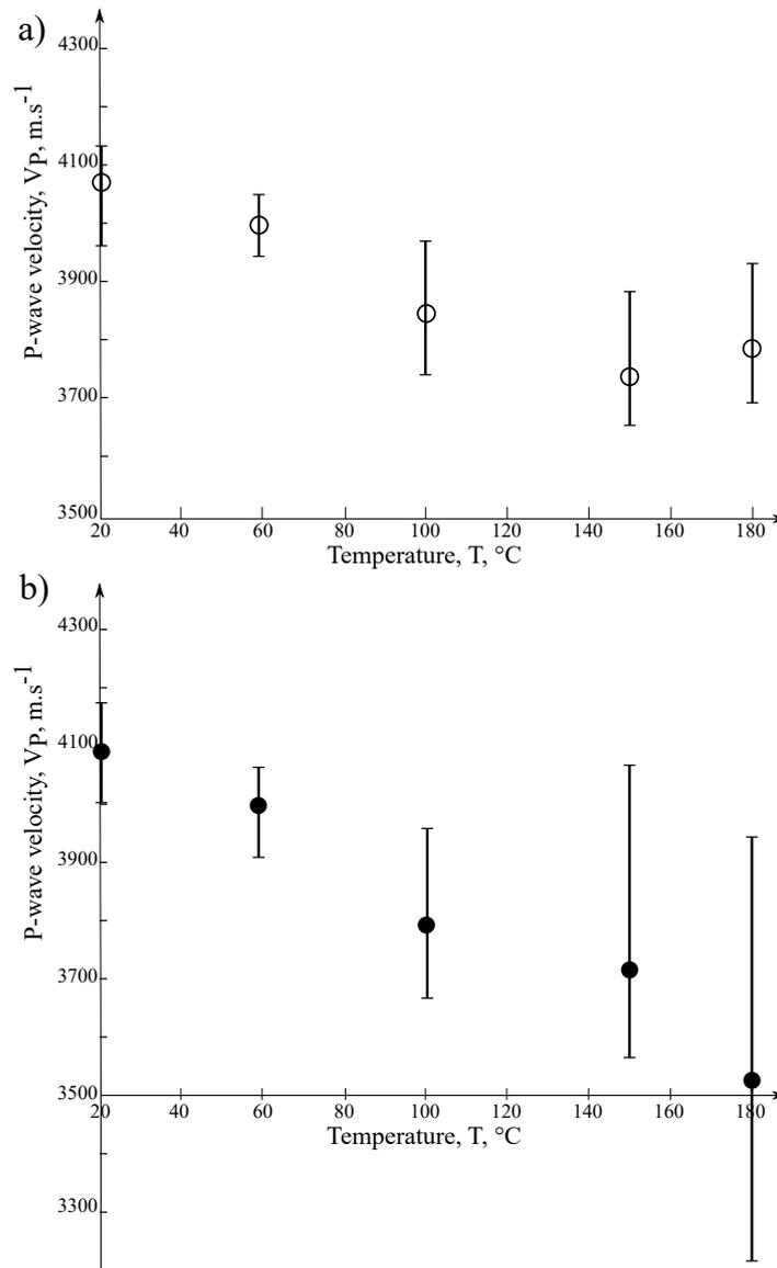
**Figure 4** P-wave velocities measured after the thermal treatments for the progressive cooling (a) and the thermal shock (b). The different samples are represented without particular differentiation but the obtained dispersion is represented with vertical bars. The dots (empty for the progressive cooling and plain for the thermal shock) are the average values obtained for each temperature.
