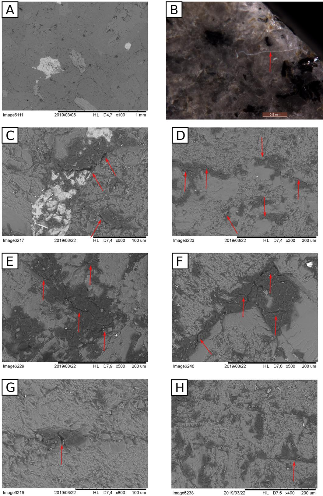
**Figure 8** Microstructural observations in our cracked samples. a) Initial state with well closed joints. b) - f) Observations made on samples after the thermal shock protocols: b) from optical microscope, on the sample boundary and c) - f) from SEM. g) - h) Observations made on samples after the progressive cooling protocols with SEM.
