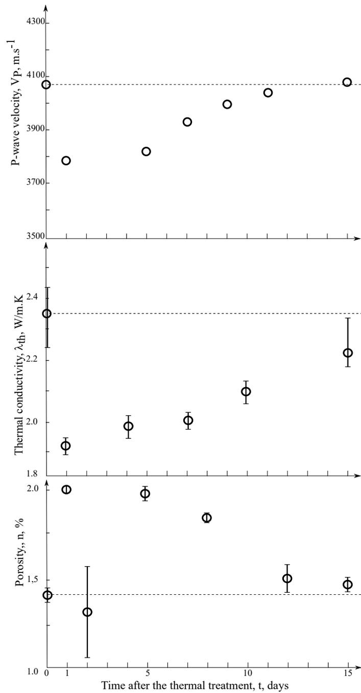
**Figure 7** P-wave velocities, thermal conductivity and porosity at the initial state (day 0), after the thermal treatment of progressive cooling (day 1) and during 15 days. Initial state are highlighted with dashed lines.
