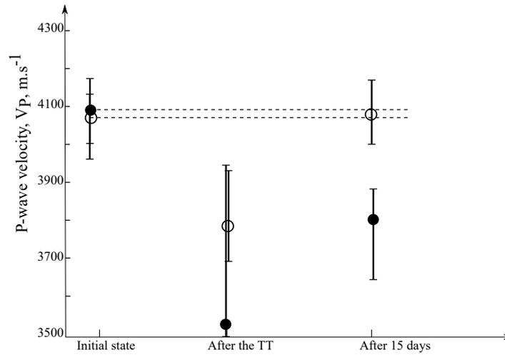
**Figure 6** P-wave velocities at initial state, measured after the thermal treatments for the progressive cooling (empty circles) and the thermal shock (plain circles), and after 15 days. Dashed lines represent the initial state for both group of 5 samples.
