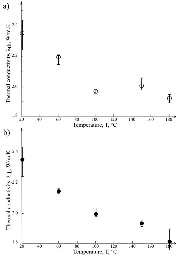
**Figure 5** Thermal conductivity measured after the thermal treatments for the progressive cooling (a) and the thermal shock (b). The main value is represented with dots (empty for the progressive cooling and plain for the thermal shock) and the obtained discrepancy between the different samples is plotted as vertical bars.
