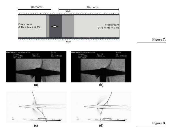
Numerical and experimental investigations of buffet dominant frequency results from the interaction between the strong shock wave and the boundary layer separation, the secondary oblique shock wave also oscillates due to the local periodic flow separation in front of the strong shock wave.
