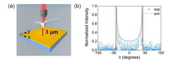
Figure 5. Far-field radiation patterns of scattered light through a 40 nm gold film on a glass substrate from a NSOM tip placed at 3 µm above the sample surface (a). (b) Normalized intensity versus the emission angle  $\theta$  in the x-z plan of the NSOM tip. Experimental data are plotted in blue and FDTD simulations in black. The vertical red line corresponds to the position of the resonance angle of excitation of leaky surface plasmons  $|\theta_{c,gold}| = 43.3^{\circ}$ .
