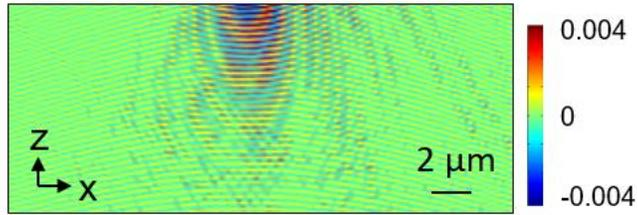
Figure S.2.: x-z section view of the wavefront reconstruction obtained experimentally by off-axis Digital Holographic Microscopy measurement of the complex EM field when the tip is 3  $\mu\text{m}$  above the metallic film, for comparison with the situation where it is in contact with it (see Figure 3.k). The figure shows  $\rho |A(x,y,z)| \cos(\phi(x,y,z))$ .
