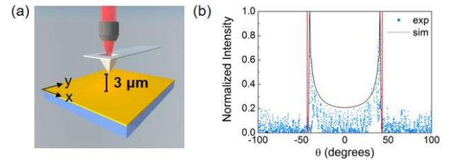
Figure 5. Far-field radiation patterns of scattered light through a 40 nm gold film on a glass substrate from a NSOM tip placed at  $3 \mu\text{m}$  above the sample surface (a). (b) Normalized intensity versus the emission angle  $\theta$  in the x-z plan of the NSOM tip. Experimental data are plotted in blue and FDTD simulations in black. The vertical red line corresponds to the position of the resonance angle of excitation of leaky surface plasmons  $|\theta_{c, \text{gold}}| = 43.3^\circ$ .
