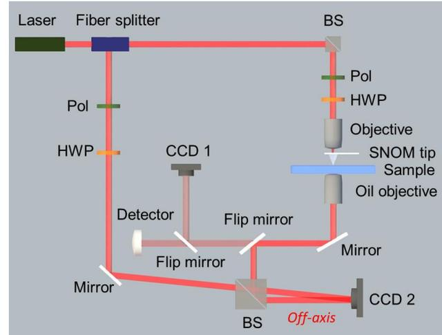
Figure 1. Schematic of the optical setup: an off-axis digital holographic microscope (DHM) is combined with a near-field scanning optical microscope (NSOM) with aperture metal-coated hollow pyramidal tip. BS: beam splitter, Pol: polarizer, HWP: half-wave plate, CCD: charge coupled device camera.
