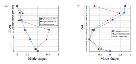
**Figure 1:** Mode shapes identification using synchronous, asynchronous and corrected data - component L: (a) 1<sup>st</sup> bending mode, (b) 2<sup>nd</sup> bending
