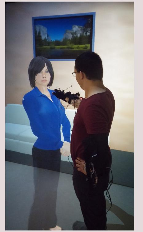
The agent's body can detect whether the human is touching the agent or not, and how (where, for how long, velocity,...), based on the spatial coordinates. However, the agent is intangible and thus we need to provide haptic feedback to make it able to touch the human.
