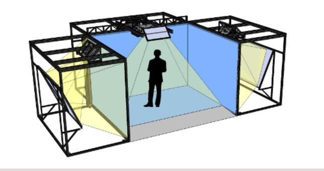
The virtual environment and the agent are projected on the walls and the floor in **stereoscopic 3D**. The user can then see everything in **1:1 scale** through the glasses.
