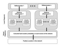
Fig. 3. Diagnosis Procedure in Wiring Networks
