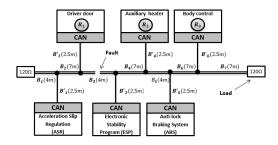
Fig. 5. A simplified CAN bus
