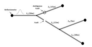
Fig. 1. Fault location ambiguity in a branched network.
