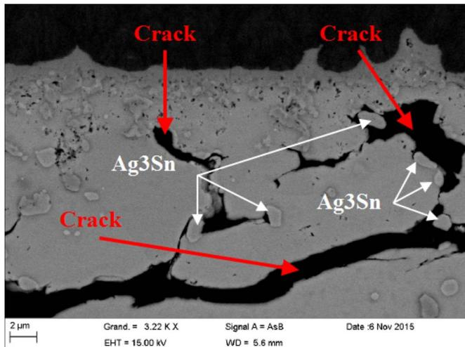
Fig. 15. Coarse Ag<sub>3</sub>Sn precipitates localized at the crack path (example of a R2512 with a corresponding damage level of 0.58).
