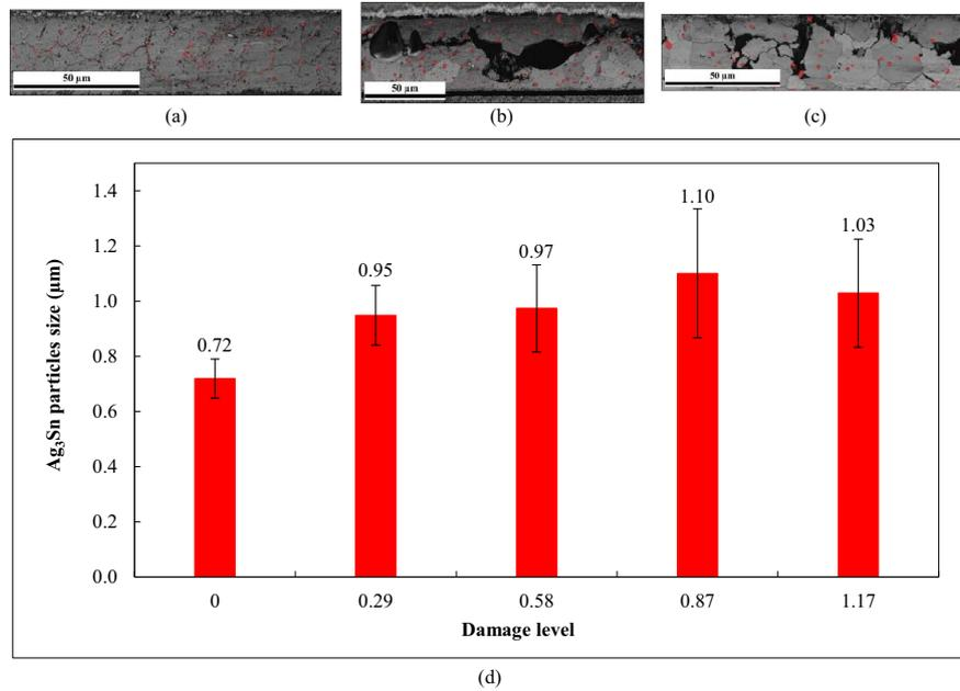
Fig. 14. Ag<sub>3</sub>Sn particles identification for a damage level of (a) 0, (b) 0.58, and (c) 1.17. (d) Evolution of Ag<sub>3</sub>Sn precipitates (colored in red on the EBSD cartography) during thermal cycling test. (For interpretation of the references to colour in this figure legend, the reader is referred to the web version of this article.)
