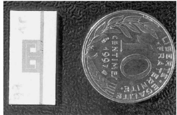
Fig. 4 : Photography of the new loop band-pass filter
