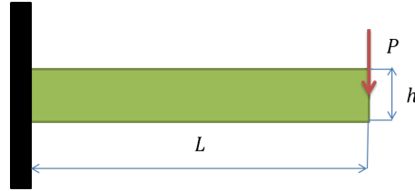
Fig. 20: Representation of the considered cantilever beam problem.
