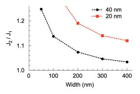
FIG. 5. Ratio between the  $J_2$  and  $J_1$  coupling strengths deduced from the micromagnetic vertex energies as a function of the width of the nanomagnets. Red squares and black dots correspond to a thickness of 20 and 40 nm, respectively.
