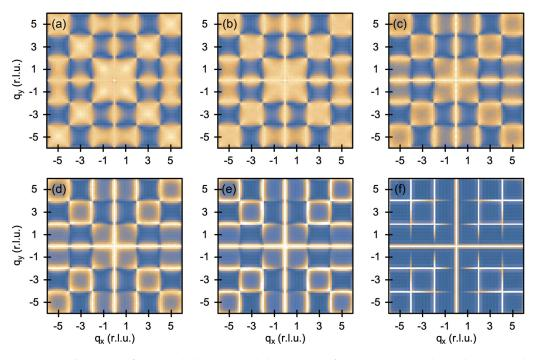
FIG. 4. Computed magnetic structure factors at the lowest sampled temperature for  $J_2 = 1$  (a), 1.01 (b), 1.03 (c), 1.05 (d), 1.1 (e), and 1.2 (f).  $J_1 = 1$  in all cases. Intensity is normalized the same way in all images. r.l.u., reciprocal lattice unit.
