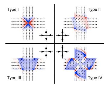
FIG. 2. Micromagnetic configurations of type-I, II, III, and IV vertices for 200-nm-wide, 20-nm-thick permalloy nanomagnets. Small black arrows represent the direction of magnetization within the nanomagnets, while the blue/red contrast codes for the divergence of the magnetization vector.
