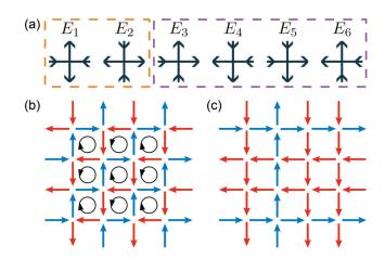
FIG. 1. (a) Schematics of the vertices involved in the six vertex model with their associated energy *E*. Because of symmetry, these vertices can be sorted in two types only (see dashed rectangles), with  $E_1 = E_2 = E_1$  and  $E_3 = E_4 = E_5 = E_6 = E_{II}$  (b). Ground-state configuration when  $E_I < E_{II}$ . (c) One given configuration belonging to the degenerate ground-state manifold when  $E_I > E_{II}$ .
