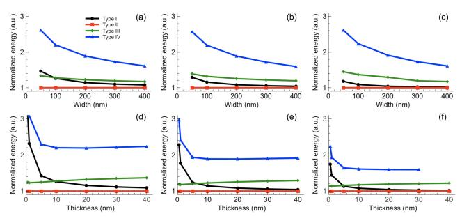
FIG. 3. Normalized micromagnetic energy of the four vertex types as a function of the width and thickness of the nanomagnets. Nanomagnets are 10-, 20-, and 40-nm-thick in (a)–(c), respectively, while they are 100-, 200-, and 400-nm-wide in (d)–(f), respectively. Type-II vertices have always the lowest energy, which is taken here as the reference energy. a.u., arbitrary units.
