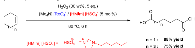
Scheme 7: Oxidative cleavage of cyclooctene and cyclohexene mediated by perhenate-containing composite ionic liquid. 67
