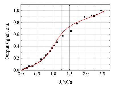
Fig. 5. Experimental (squares, normalized value  $A_D \sim \int dt \sqrt{U_D(t)}$  where  $U_D(t)$  is the detector signal) and theoretical (red line,  $\langle \theta_e^2(r_m) \rangle^{1/2}$  from Eq. (14)) dependences of a single pulse area after the resonant medium as a function of the incoming pulse area, corresponding to the McCall-Hahn area theorem.
