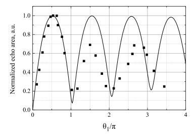
Fig. 8. Experimental (squares, normalized  $A_D \sim \int \sqrt{U_D} dt$ ) and theoretical  $(\langle \theta_e^2(r_m) \rangle^{1/2})$  from Eq. (14) with  $r_0 = 97 \mu \text{m}$ ,  $r_m = 25 \mu \text{m}$ ) dependencies of primary photon echo signal on the first incoming pulse area  $\theta_1(0,0)$  with constant  $\theta_2(0,0) = 1.1\pi$ . See text for details.
