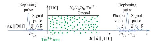
Fig. 1. The classic two pulse echo sequence propagation through the  $\mathrm{Tm}^{3+}$  doped crystal.  $\vec{k}$  is the common wave vector of three pulses parallel to the external magnetic field. The first signal pulse is partly absorbed by the medium, the second pulse triggers the rephasing process which results in the photon echo emission.
