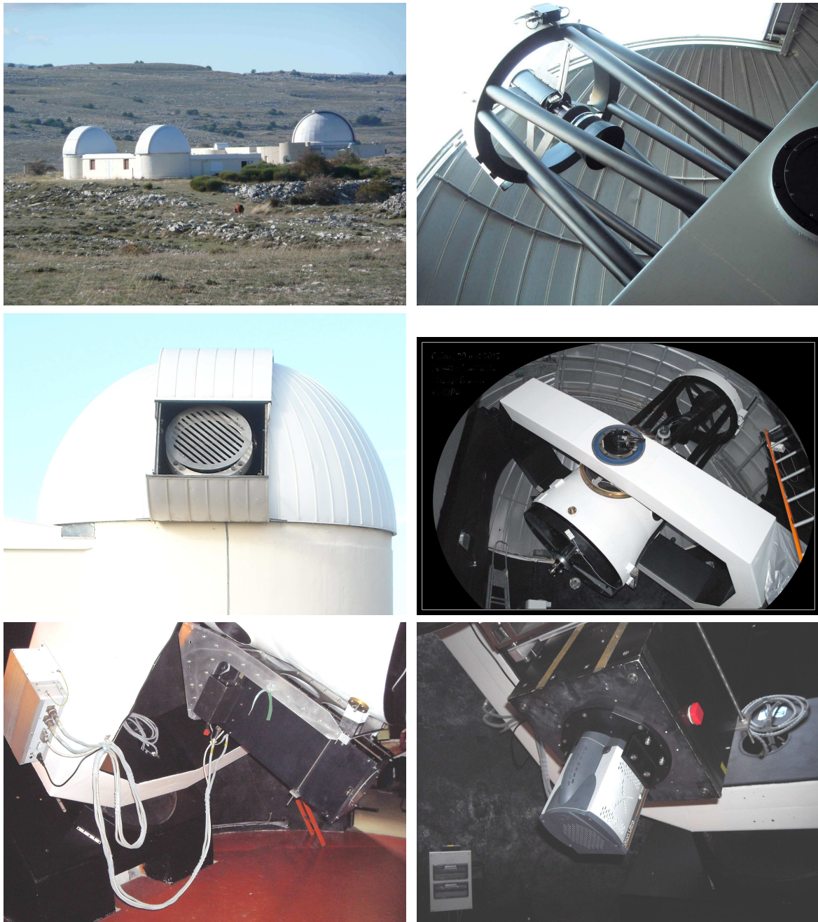
Fig. 1 Photographs of PISCO mounted on the 1-m Epsilon telescope in Calern. From top to bottom and left to right: overview of the observatory (the Epsilon telescope dome is the central one), upper part of the telescope, grating mask fitted on top of the telescope during scale calibration, telescope before the installation of the instrument (May 2015), PISCO mounted on the side of the telescope tube, EMCCD Andor iXon Ultra 897 camera attached to PISCO.
