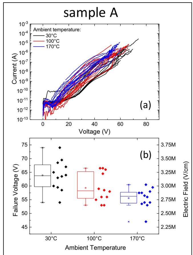
**Fig. 3.** (a) Current-voltage characteristics of the devices on sample A at different ambient temperature (i.e.  $30^\circ\text{C}$ ,  $100^\circ\text{C}$  and  $170^\circ\text{C}$ ). (b) Box chart of the failure voltages of the tested device of sample A. Right y-axis shows the corresponding electric field.
