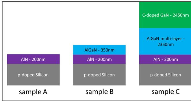
**Fig. 1.** Schematic representation of the three tested samples. Sample A (left) consists of 200 nm thick layer of AlN grown on a conductive ( $1 \cdot 10^{19} \text{ cm}^{-3}$  boron-doped) silicon substrate. Sample B (center) has an additional 350 nm thick AlGaN layer. Sample C (right), over the AlN nucleation layer, has a 2350 nm thick strain-relief layer and a 2450 nm carbon doped ( $2 \cdot 10^{19} \text{ cm}^{-3}$ ) GaN layer.
