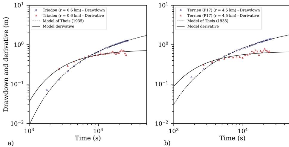
Fig. 5. Diagnostic plots of daily drawdown monitored at a) Triadou and b) Terrieu (P17) boreholes and its logarithmic derivative for the daily pumping cycle in June 20, 2012 (Fig. 3). The model of Theis (1935) is represented by a black dashed line for the drawdown curve and by a continuous black line for the derivative curve.
