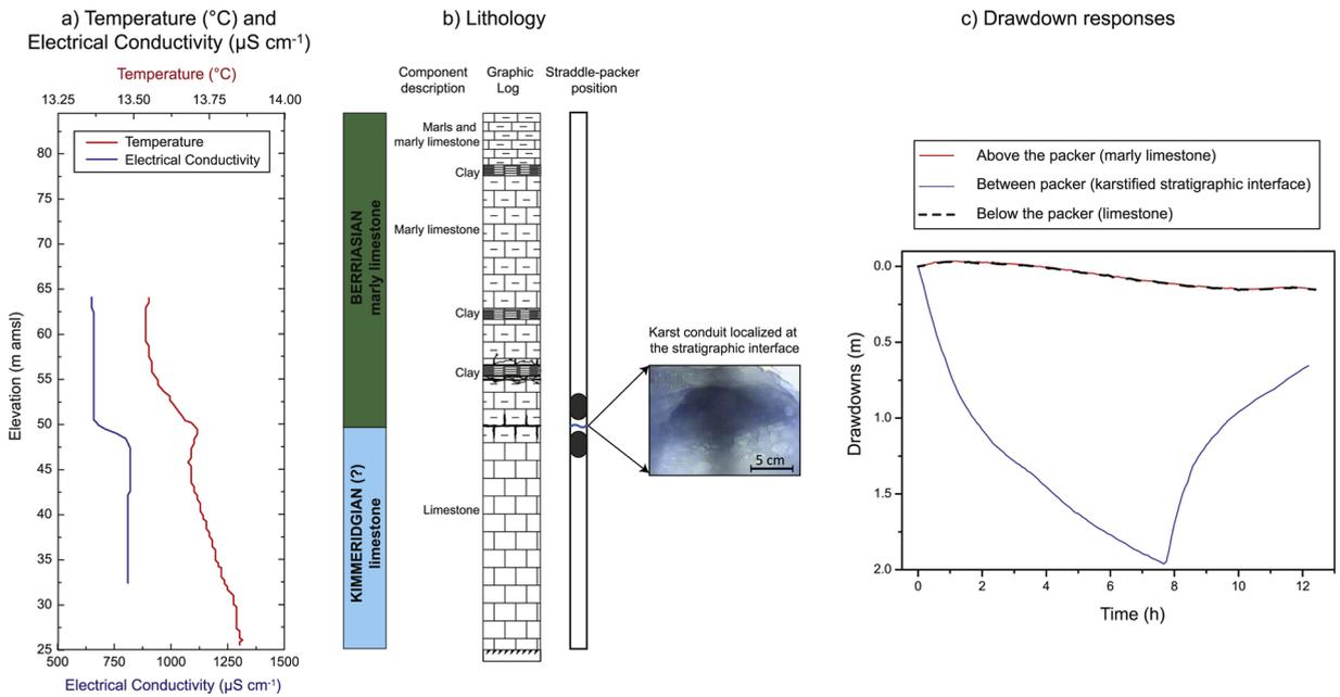
**Fig. 10.** Main karstic flow paths into borehole P15: location of the preferential flow path using a) The temperature and electrical conductivity logs; b) Lithology log from interpretation of drill cuttings (modified from Pitard, 1976) with position of the straddle-packer isolating the karst conduit at 50 m amsl; c) Drawdown responses in P15 above, between and below the straddle-packer in response to pumping at the Lez station.
