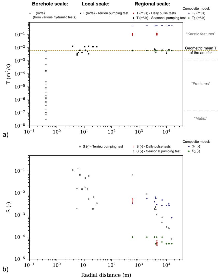
**Fig. 12.** Synthesis of hydraulic parameters of the Lez aquifer estimated at borehole scale (Table 5), local scale (Table 4) and regional scale (Tables 3 and 2 and 1): a) Transmissivity, b) Storativity.
