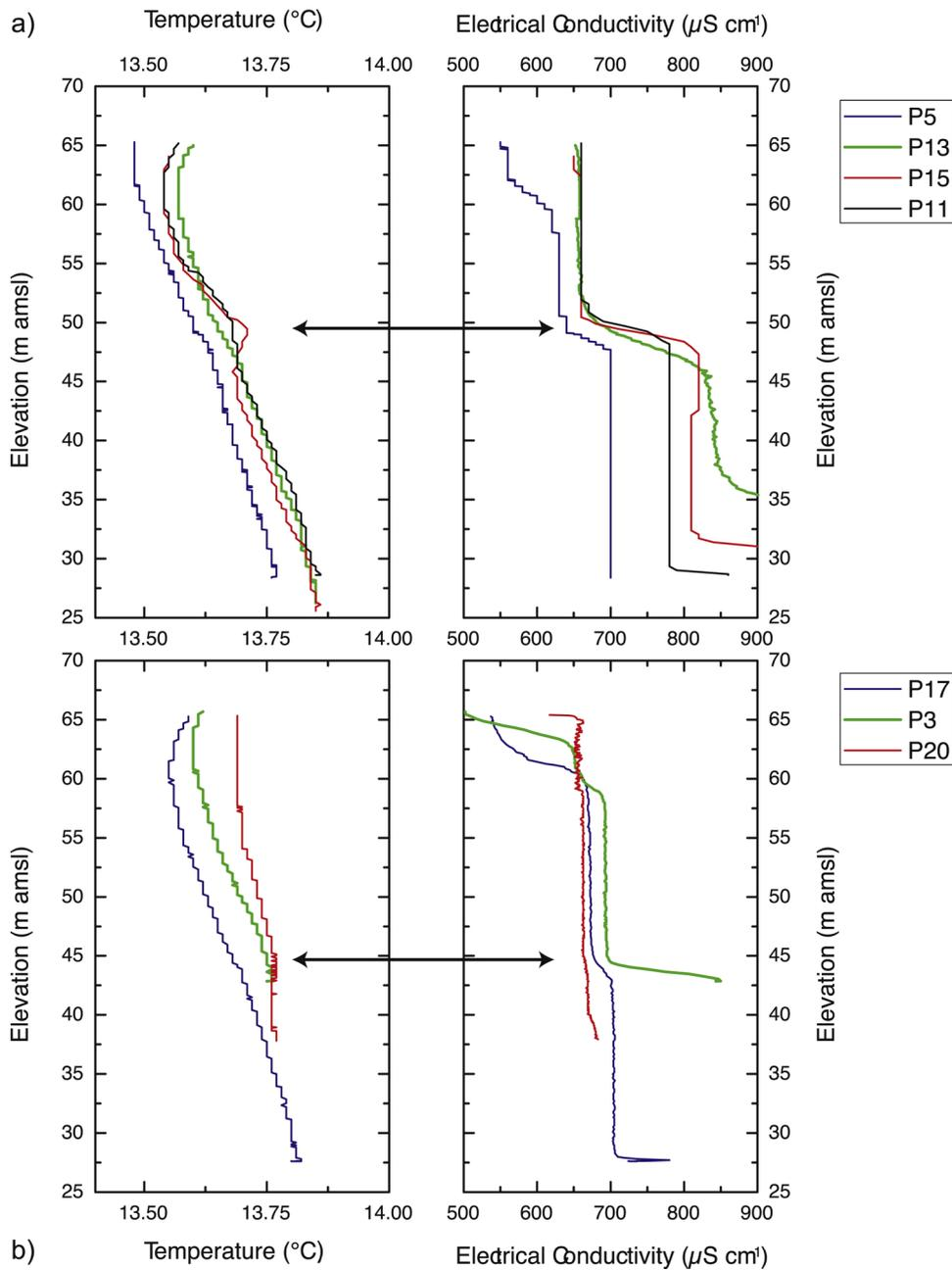
**Fig. 9.** Temperature and electrical conductivity logs in the P5, P13, P15, P11 boreholes at the Terrieu experimental site, made in June 2012 (a) and February 2013 (b). The main flow zone appears to be located between 45 and 50 m amsl (black arrows).
