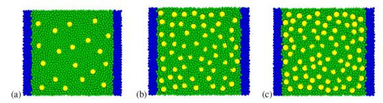
**Fig. 30.** Geometry of specimens using three fiber volume fractions: (a)  $V_f = 0.1$  (b)  $V_f = 0.3$ ,(c)  $V_f = 0.4$ .
