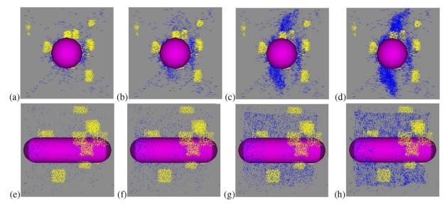
**Fig. 28.** Failure process for  $P_r = 2\%$  and  $\sigma_M | \sigma_I = 0.5$ . Broken bonds in matrix (blue color) for different macroscopic values of strain: (a,e)  $\varepsilon = 14.10^{-3}$ , (b,f)  $\varepsilon = 16.10^{-3}$ , (c,g)  $\varepsilon = 17.10^{-3}$ , (d,h)  $\varepsilon = 19.10^{-3}$  displayed in (a,b,c,d) face views and (e,f,g,h) side views.
