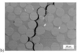
Fig. 2. Fiber-matrix debonding: section perpendicular to the fiber axis [3].
