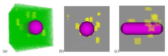
**Fig. 26.** Configuration of defaults (yellow beam) in specimen for  $P_r = 2\%$  displayed (a) in 3D (b) in face views (c) in side views (For interpretation of the references to color in this figure legend, the reader is referred to the web version of this article.).
