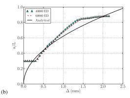
Fig. 14. (a) Load-displacement curves and (b) crack length—displacement curves in the DCB test.
