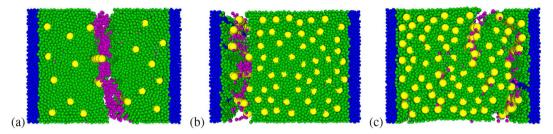
Fig. 31. Crack path in composite specimen for  $\sigma_M/\sigma_I=2$  at strain  $\varepsilon=0.184$  for (a)  $V_f=0.1$ , (b)  $V_f=0.3$  (c)  $V_f=0.4$ .
