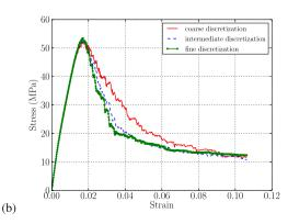
Fig. 20. Stress-strain curves for the three specimens (a) using BBF criterion (b) using RDEF criterion.
