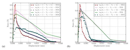
**Fig. 33.** Compare the evolution of force-displacement curve with FEM [1] at  $V_f = 0.1$ ,  $V_f = 0.3$  and  $V_f = 0.4$  for (a)  $\sigma_M/\sigma_I = 2$  and (b)  $\sigma_M/\sigma_I = 0.5$ .
