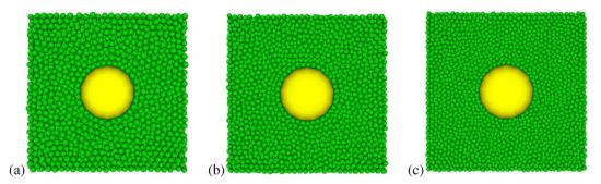
Fig. 19. Single-fiber composite specimens (a) coarse discretization (18835 ED), (b) intermediate discretization (27916 ED) (c) fine discretization (46004 ED).
