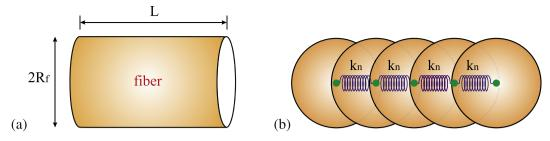
Fig. 18. Fiber modeling: continuous medium (a) and the spring link connected the DE of fiber in DEM (b).
