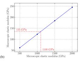
**Fig. 13.** Calibration curves for present material. (a) Radius ratio  $\tilde{r_{\mu}}$  calibration and (b) microscopic Young's modulus  $E_{\mu}$  calibration.
