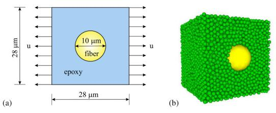
Fig. 17. Configuration of single-fiber test in (a) continuous media (b) discrete media.
