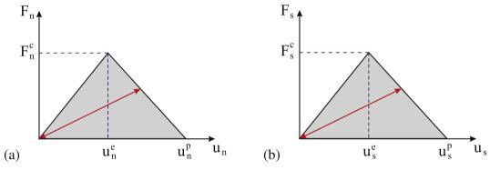
Fig. 8. Constitutive behavior of contact softening model (a) normal contact (b) shear contact.
