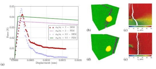
**Fig. 23.** (a) Compare the evolution of force-displacement with the Finite Element Modeling [1] for  $\sigma_M/\sigma_I = 2$  and  $\sigma_M/\sigma_I = 0.5$ , Crack path for (b)  $\sigma_M/\sigma_I = 2$  and (c) the equivalent in FEM, (d) for  $\sigma_M/\sigma_I = 0.5$  and (e) the equivalent in FEM.
