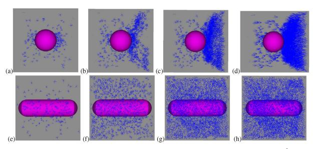
**Fig. 25.** Failure process for  $\sigma_M/\sigma_l = 0.5$ . Representation of the broken bonds in matrix (blue color) for different macroscopic values of strain. (a,e)  $\varepsilon = 14.10^{-3}$ , (b,f)  $\varepsilon = 17.10^{-3}$ , (c,g)  $\varepsilon = 35.10^{-3}$ , (d,h)  $\varepsilon = 53.10^{-3}$ . With face views (a,b,c,d) and side views (e,f,g,h) (For interpretation of the references to color in this figure legend, the reader is referred to the web version of this article.).
