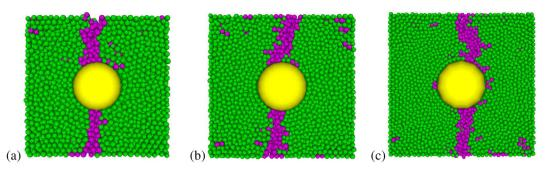
Fig. 21. Path of the crack,  $\varepsilon = 0.018$ , using BBF criterion (a) with the coarse discretization (b) with the intermediate discretization (c) with the fine discretization.
