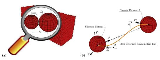
Fig. 3. Illustration of the cohesive beam bond in GranOO [42].
