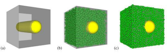
Fig. 5. Filling procedure for mono-fiber composite, V = 0.1 (a) pre-filling stage, (b) intermediate stage and (c) final compacted domain.
