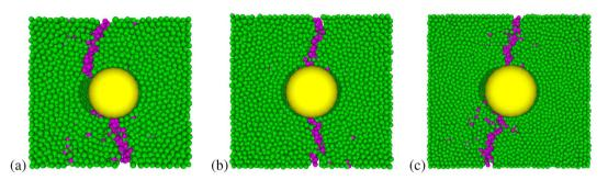
Fig. 22. Path of the crack,  $\varepsilon = 0.08$ , using RDEF criterion (a) with the coarse discretization, (b) with the intermediate discretization and (c) with the fine discretization.
