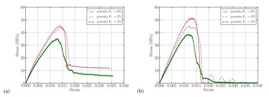
**Fig. 27.** Evolution of stress-strain for  $P_r = 0\%$ ,  $P_r = 2\%$  and  $P_r = 5\%$  with: (a)  $\sigma_M/\sigma_I = 2$  (b)  $\sigma_M/\sigma_I = 0.5$ .
