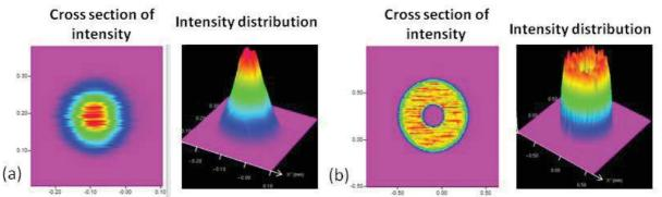
Figure 2: Intensity distributions at the focal point with (a) the 100  $\mu$ m core fiber (500 W,  $\Phi$ =150  $\mu$ m), (b) the 400  $\mu$ m outer fiber (500 W,  $\Phi$ =150  $\mu$ m) measured with a Primes Focus monitor device.
