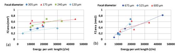
Figure 3: Fusion zone area as a function of energy per unit length for different focal diameters, (a) with the core fiber, (b) with the outer fiber.
