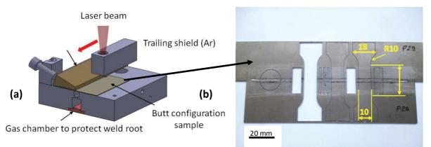
Figure 1: Experimental set-up, (a) Laser welding fixture, (b) localization of metallographic and tensile test sample.
