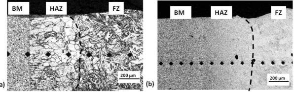
Figure 7 : Welds made at 1500 W, 4.5 m/min, diam. 370 µm (a) CP Ti grade 2, (b) Ti-6Al-4V alloy.
