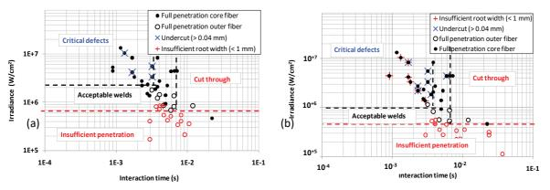
Figure 6: Relationship between weld full penetration, laser power density and interaction time, (a) CP grade 2 titanium, (b) Ti-6Al-4V titanium alloy
