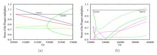
Figure 9: Variation of the spectrum (norm of the main Floquet multipliers) with Gr for (a) the limit cycle with all the symmetries and (b) the limit cycle with the  $S_c$  symmetry. Solid (dashed) lines are used for steady (complex conjugate) Floquet multipliers. The associated modes have all the symmetries (red line), the  $S_l$  symmetry (blue line), the  $S_c$  symmetry (green line), the  $S_{\pi}$  symmetry (yellow line) or no symmetry (pink line). The results are for Pr = 0.005.
