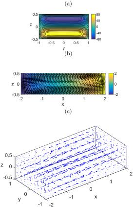
Figure 2: For Pr = 0.025 and  $Gr = 3 \times 10^4$ : (a) Longitudinal velocity field u(y, z) in the  $V_t$  plane; (b) Velocity vector (u, w) and temperature  $-2 \le \Theta(x, z) \le 2$  fields in the  $V_t$  plane; (c) A three dimensional visualisation of the velocity vector field showing the circulation loop in the cavity.
