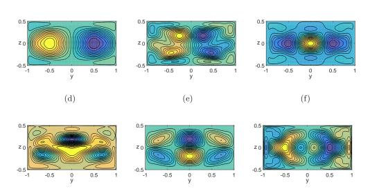
Figure 5: Contours of the longitudinal velocity perturbation u'(y,z) in the transverse  $V_t$  plane for the critical modes (real part) associated with different bifurcation points. The sub-figures (a)-(f) correspond to  $H_{c,25}^P$  at Pr=0.025,  $H_{w,25}^S$  at Pr=0.015,  $P_l^P$ ,  $H_l^S$  and  $H_a^P$  at Pr=0.005 and finally  $H_{c,0}^P$  at Pr=0, respectively.
