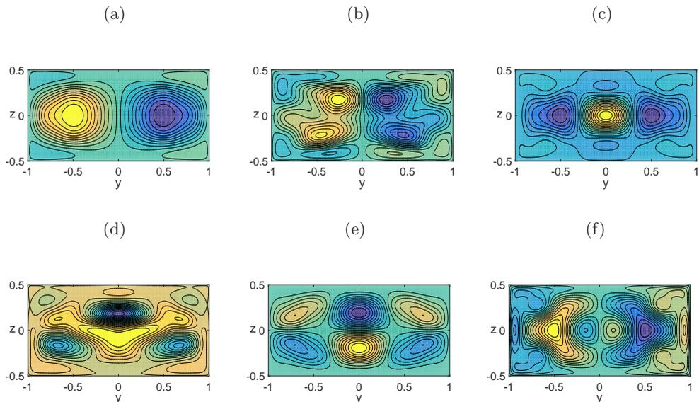
Figure 5: Contours of the longitudinal velocity perturbation  $u'(y, z)$  in the transverse  $V_t$  plane for the critical modes (real part) associated with different bifurcation points. The sub-figures (a)-(f) correspond to  $H_{c,25}^P$  at  $Pr = 0.025$ ,  $H_{w,25}^S$  at  $Pr = 0.015$ ,  $P_l^P$ ,  $H_l^S$  and  $H_a^P$  at  $Pr = 0.005$  and finally  $H_{c,0}^P$  at  $Pr = 0$ , respectively.
