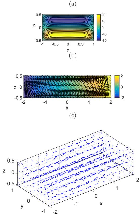
Figure 2: For  $Pr = 0.025$  and  $Gr = 3 \times 10^4$ : (a) Longitudinal velocity field  $u(y, z)$  in the  $V_t$  plane; (b) Velocity vector  $(u, w)$  and temperature  $-2 \leq \Theta(x, z) \leq 2$  fields in the  $V_t$  plane; (c) A three dimensional visualisation of the velocity vector field showing the circulation loop in the cavity.
