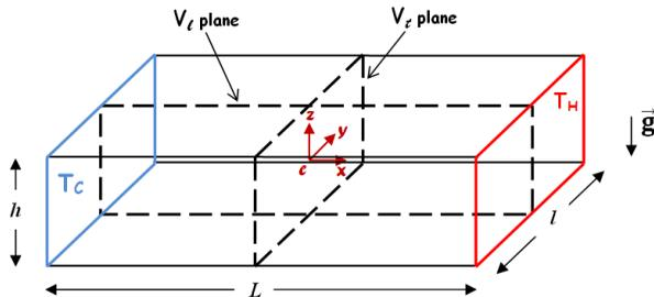
Figure 1: Geometry of the differentially heated cavity. The endwalls located at  $\bar{x} = -L/2$  and  $\bar{x} = L/2$  are held at fixed temperatures  $T_C$  and  $T_H$  (with  $T_H > T_C$ ), respectively, whereas the sidewalls are insulating boundaries.
