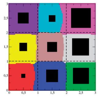
**Figure 7.** Illustration of the influence surfaces (colored areas) associated with each pore (black filled square) at the surface. The dashed lines delineate the boundary of each cell at the surface. The influence surface area of a pore is the surface area of the pore together with the area of the colored surface surrounding the pore. The stairs at the boundary between two influence surfaces are due to the discrete method used to determine the boundary.
