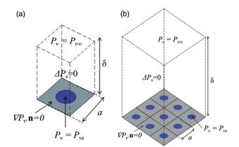
Figure 1. Computional domains: (a) single unit cell and (b)  $3 \times 3$  square arrangement of wet surface pores.
