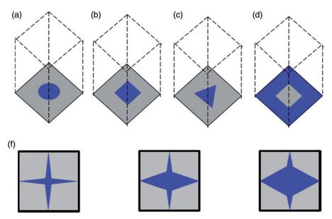
**Figure 2.** The various surface elementary pore shapes (wet zone in blue, solid surface in grey): (a) circular, (b) square, (c) triangle, (d) square complement, and (e) Star shapes corresponding to  $\theta = 0.1$ ,  $\theta = 0.2$ , and  $\theta = 0.3$ , respectively.
