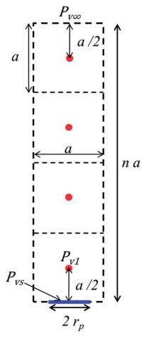
**Figure A1.** Finite volume distribution in the external diffusive mass boundary layer used to obtain Eq. (A-5). The thick blue line materializes the wet pore at the surface. The red dots correspond to the computational points.
