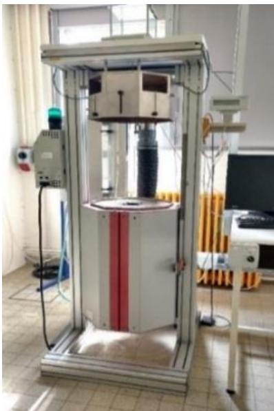
Figure 3. Large scale simultaneous TGA-DTA instrument built at INERIS.
