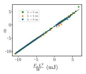
FIG. 4. Dimensionless parameter  $\alpha$ , computed numerically, as function of  $F_x L^2/W$ , measured experimentally. The value of  $B=1.07 \mathrm{mJ}$  is inferred from the inverse of the slope of the linear fit represented by the solid line.
