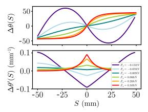
FIG. 5. Local deformation  $\Delta\theta(S)$  and its derivative  $\Delta\theta'(S)$  as functions of the curvilinear coordinate S. These curves are obtained using the profiles computed numerically for different values of the force  $F_x$ .
