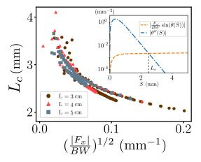
FIG. 6. Critical length scale  $L_c$  as defined by Eq. (17) as a function of the inverse length  $(|F_x|/BW)^{1/2}$  for different values of L. Inset: log-lin curve of the absolute value of each term in Eq. (9) with  $\beta = 0$  near the crease for  $F_x = -0.092$ N.
