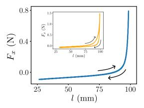
FIG. 2. Mechanical response of a folded mylar sheet during the first unfolding-folding cycle. Here, l is the distance between the clamps and  $F_x$  is the applied force. The main figure corresponds to an annealed sample while the inset shows the same sample before annealing. The arrows indicate the direction of the displacement of the upper clamped edge.
