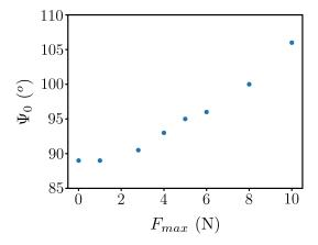
FIG. 8. Rest angle  $\Psi_0$  as function of the maximal vertical force  $F_x$  reached while stretching the fold. We increase l until  $F_x = F_{max}$  and lock it for one minute. Then, we release the sample and let it relax for one minute before taking a photo of the rest shape to recover  $\Psi_0$  as done previously.
