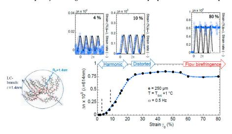
**Figure 3.** Strain dependence of the birefringent signal (peak value of the signal) in the isotropic phase of the 12-units liquid crystal (T-TS<sub>AI</sub> = +1 °C, quartz substrate) at 0.5 Hz. The strain amplitude is the maximum displacement length  $\delta l$  divided by the sample thickness ( $\gamma_0 = \delta l/e$ ).
