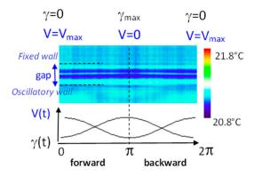
**Figure 15.** Polymer slab of 0.185-mm-thickness under oscillatory strain: the melt exhibits non-uniform temperatures with the emergence of cold thermal bands (dark blue) coexisting upon applying an oscillatory shear stress of ( $\gamma = 1200\%$ ,  $\omega = 2 \text{ rad/s}$ ). The bottom curves illustrate the strain and the velocity over a period. Complementary information is available in references [58,59].
