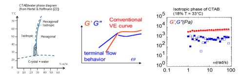
**Figure 12.** Using total wetting conditions, the liquid phase (dilution 18%) of salt-free CTAB-water (Cetyl TrimethylAmmonium Bromide solution) measured at 33 °C (isotropic phase) and the 0.300-mm gap thickness exhibit solid-like behavior with G' independent of the frequency and exceeding G" [51].
