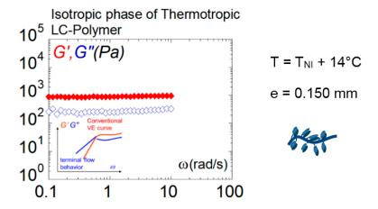
**Figure 8.** A strong solid-like response is measured above the isotropic–nematic transition by a liquid crystal polymer (viscoelastic moduli  $G'(\blacklozenge)$ ,  $G''(\lozenge)$  recorded at 14 °C above the transition and 0.150 mm gap thickness). The lower inset displays for comparison the conventional polymer melt behavior fulfilling the Maxwell model [32]). From Mendil, Noirez, Baroni 2006 [36]). With kind permission from The European Physical Journal (EPJ).
