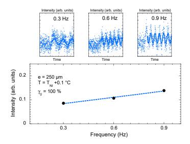
**Figure 5.** Optical response (transmittance intensity) measured upon applying a low-frequency mechanical strain in the isotropic phase of 4-octyl-4'-cyanobiphenyl (8CB) (T - T<sub>NI</sub> = +0.1 °C, quartz substrate, strain rate  $\gamma_0$  = 100%). The transmittance displayed at  $\omega$  = 0.3 Hz, 0.6 Hz and 0.9 Hz is weak. Device limitations do not enable a conclusive analysis (top figure).
