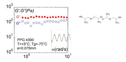
**Figure 13.** Frequency dependence of the elastic  $G'(\omega)$ : • and viscous moduli  $G''(\Box)$ : □, measured for a glass former liquid (polypropyleneglycol (PPG4000),  $M_W = 4000$ , Tg = -75 °C) at T = +5 °C (0.075 mm gap thickness–alumina plate-plate fixtures). The insert shows the superposition of the strain (green points) and the stress (red points) waves highlighting the instant response of the liquid.
