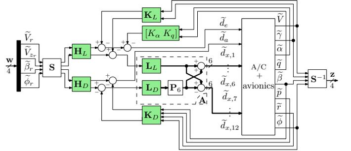
Fig. 3. The longitudinal/lateral closed-loop control block diagram.
