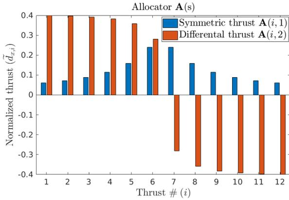
Fig. 5. Bar-diagram of the allocation matrix  $\mathbf{A}$ .
