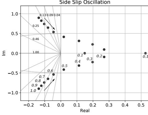
Fig. 2. Evolution of the eigenvalues of the side slip oscillation of the reference aircraft with the reduction of the vertical tail surface area, from  $S_v/S_{v_0} = 1$  to  $S_v/S_{v_0} = 0.1$ . The number in italic next to an eigenvalue indicates the corresponding quantity  $S_v/S_{v_0}$ . The regular number next to a dashed line corresponds to the damping value.
