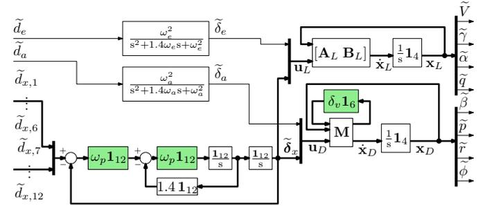
Fig. 4. The A/C + avionics block diagram.
