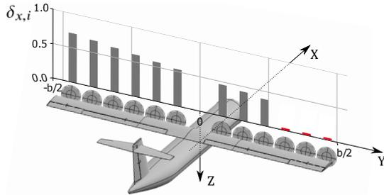
Fig. 1. Illustration of thrust distribution on the reference aircraft with twelve electric engines.
